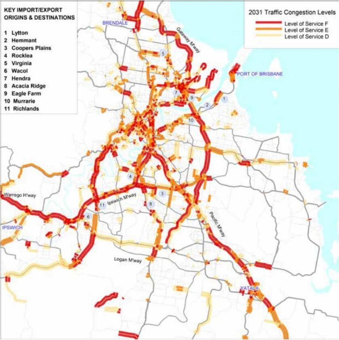
FIGURE 28: ACCESS TO PORT OF BRISBANE: ESTIMATED LEVEL OF SERVICE FOR BRISBANE AND ADJACENT REGIONS FOR 2031 SOURCE: PORT OF BRISBANE, 2013
