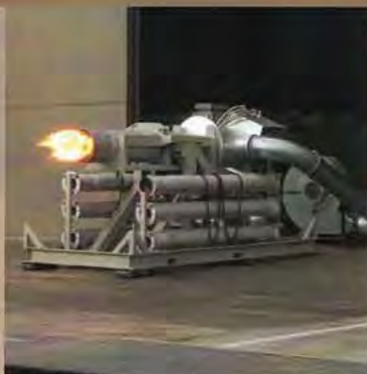
Low NOx Recirculated Combustion Gas Burner System.
